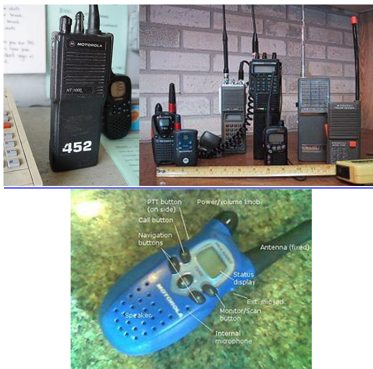
Figure 8. Portable radio transceiver( http://en.wikipedia.org/wiki/Walkie-talkie )
