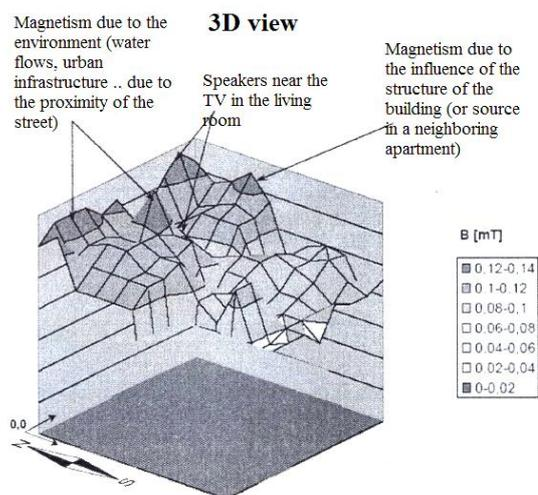
Figure 3. An example of the results and analysis of measurements of static EM fields
